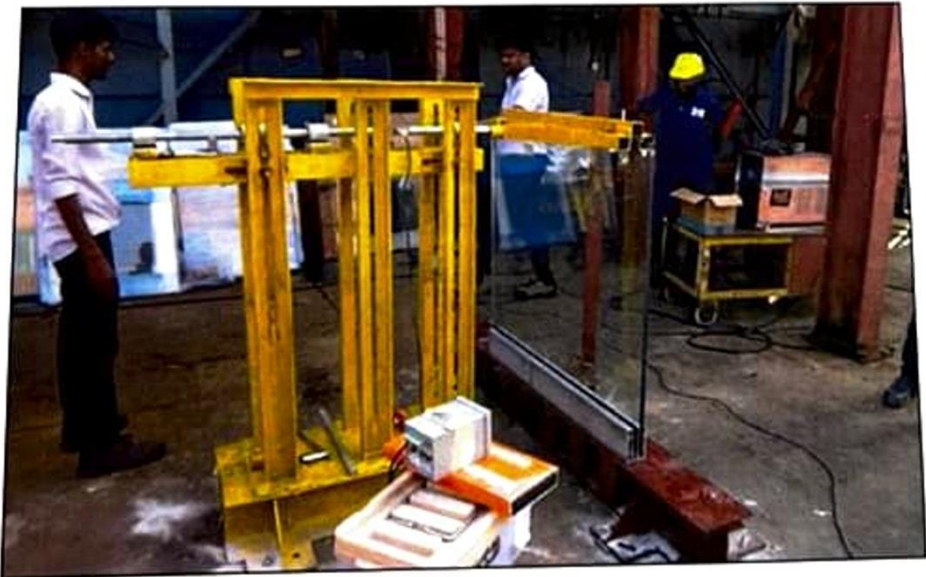
Photo (2) - Stainless steel reaction frame for uniform load test
