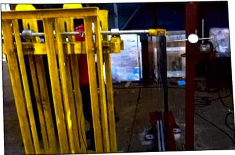
Photo (3) - Stainless steel reaction frame for concentrated load test
